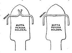
and never between the surface of the one and the transverse section of the other. In order to ensure this result, the two pieces of nerve should be laid on the gutta-percha holder, so as to establish the contact either of their surfaces or of their transverse sections on the middle of the holder, while the two opposite extremities of the nerves hang down over the two opposite sides of the holder.
